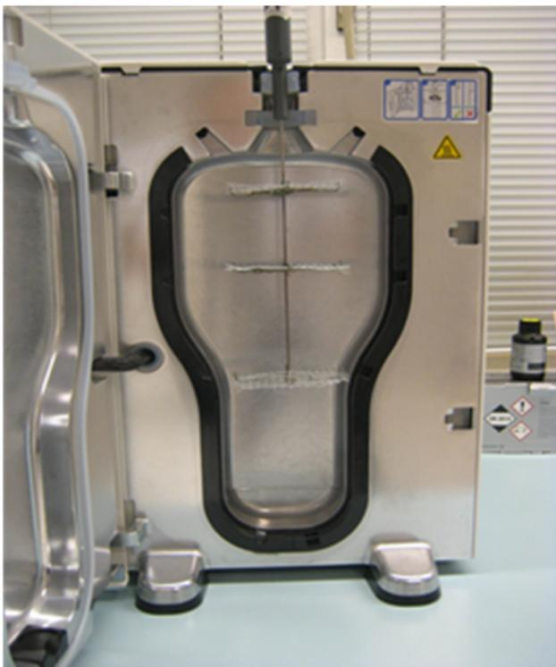
**Figure 1:** Automated testing device with stainless steel discs contaminated with test virus suspension. Three carriers with virus were run in parallel. A fourth carrier without virus is measuring the cytotoxicity in the test system.
