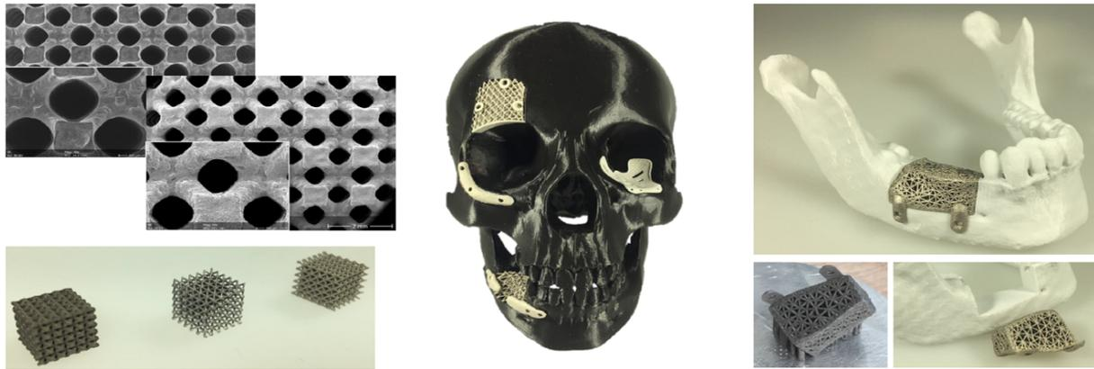
Figure 12: 3D printing of magnesium implants using selective-laser-melting (SLM)
