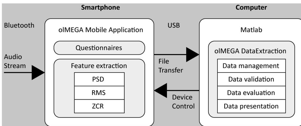
Figure 1: System modules and interaction
