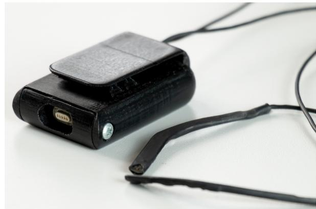
Figure 6: Bluetooth transmitter box with miniature microphones
