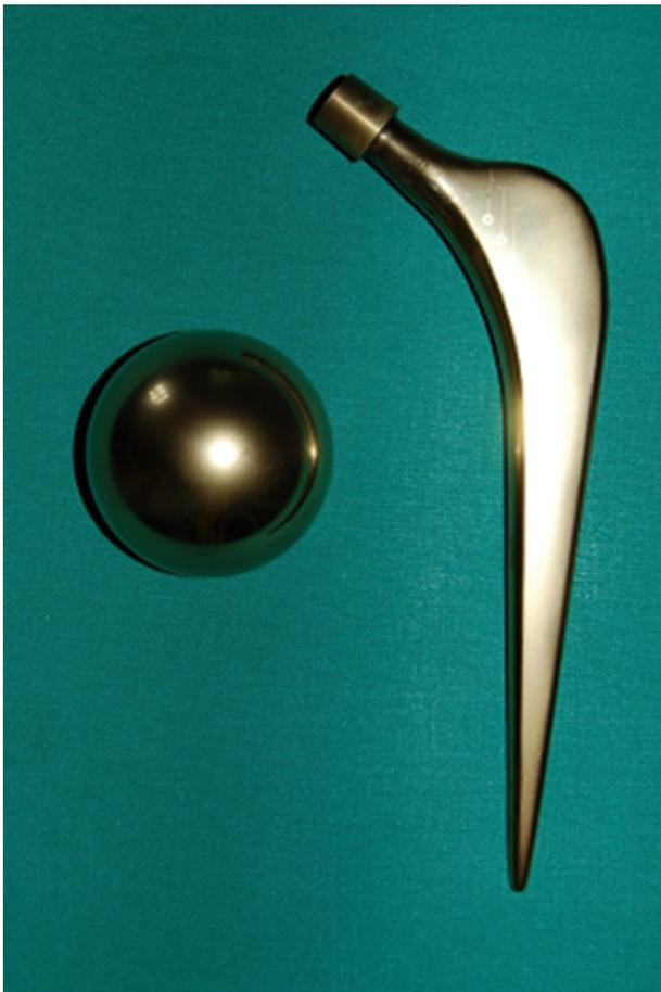
**Figure 1:** TiCuN coated (DOT GmbH, Rostock, Germany) hip stem and jumbo head for a hemiarthroplasty
