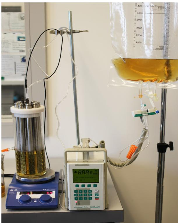
**Figure 1: Experimental setup.** On the left European Biofilm Reactor (EUREBI) with vertical placed titanium discs, on the right infusion bag as storage vessel for liquid culture, in the middle Infusomat to control the flow of liquid culture.
