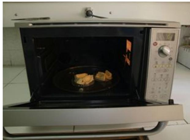
Figure 2: Microwave set with inoculated stone casts prepared for irradiation
